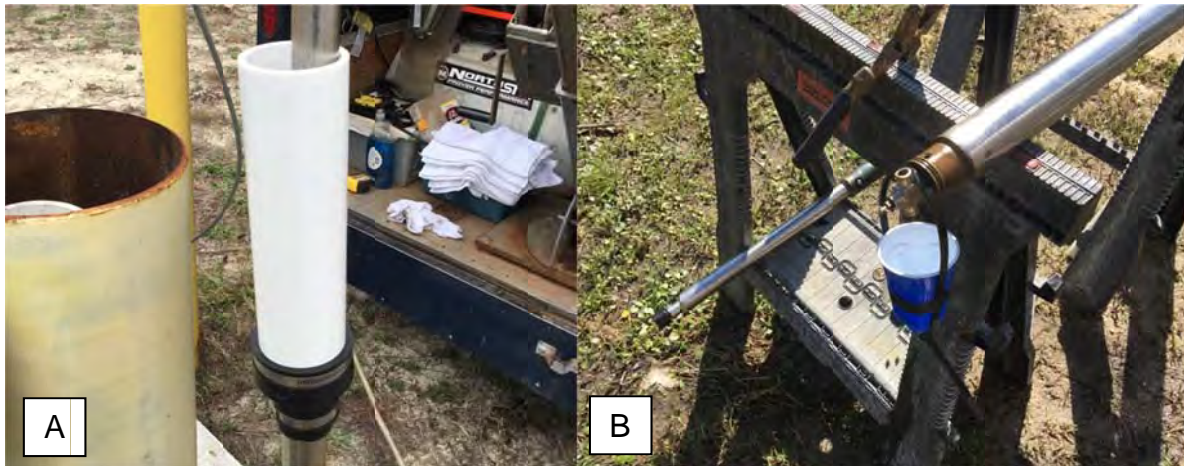
Figure 4. RMBAKER water sampling jigs. Photo A shows the jig for capturing sample blanks. Photo B shows the jig for holding sample bottles while discharging the sample from the vacuum chamber.
